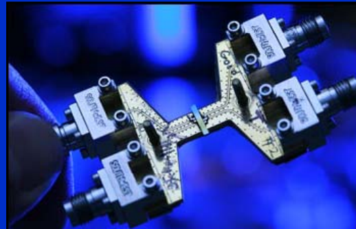
Charge-Injected Silicon (Intel) Speed: 40 GHz (2007) Drive voltage: 4 V Insertion loss: 19 dB
